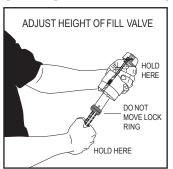
The valve height should be adjusted so that the critical level mark "C.L." on the valve is located at least 25mm. ABOVE the overflow outlet. The 400UK valve can be adjusted from 225mm. to 350mm. to fit most cisterns by TWISTING THE SHANK in or out of the valve body.
