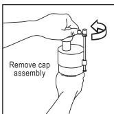
5. Make sure water supply is off. With RIGHT HAND push float cup up. (See drawing) Hold valve shaft tight.
