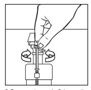
8. Turn on water supply. Submerge the FLOAT CUP under the water for 30 seconds. Adjust the water to desired level by turning WATER LEVEL ADJUSTMENT ROD and moving FLOAT CUP up or down. Water level should be set approximately 25mm. below overflow outlet or to water line on cistern.
