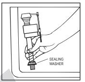
2. Place sealing washer on threaded shank and position valve in cistern, passing threaded shank through hole
