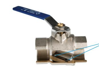
Two internal drain holes in the ball avoid the build up of pressure caused by frosted water.
