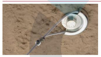
A structural attachment that maximizes the load capacity on a post-installed concrete anchor by neutralizing the prying effect from the cable load. This increases the allowable design load per anchor and results in the need for fewer bracing locations.
