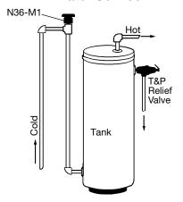
Figure 2 **Domestic Hot Water Supply Tanks** and Heaters with Bottom Feed
