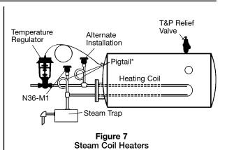
\*Note: When used for steam service, be sure to use pigtail to prevent live steam from damaging N36 valve.
