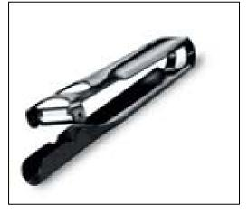
This tool is available from the Rain Bird GSP Production and Service Center at (520) 434-6208 using part number GSP 700404. Tools such as utility, pocket, carpet, and box cutter knives should not be used nor should Romex strippers. Damage to the inner insulation will invariably occur with these tools and could negatively impact system performance.
