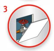
Align panel's inside ledge with bottom of opening, then push panel against wall. To remove, simply pull out at opposite corners. NOTE: If the panel will be used frequently, paint the raw edges of the wall/ceiling with latex or oil-based paint for greater durability.
