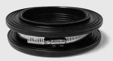
Fernco Puddle Flanges are installed during construction to seal around the outside of pipes that are required to pass through concrete structures, such as tanks, manhole chambers, shafts, floor slabs and basements.
