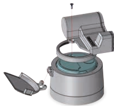
Picture 4: Mounting of the EDC-C.
