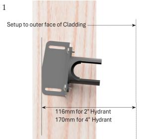
The hydrant should be set up so that the back of the cap assembly will be hard against the cladding when installed. Care should be taken to position the outer flange in a position that suits the profile of the cladding. For example, where vertical weatherboards are being used, the outer flange should be positioned in the center portion of the board, so it doesn't interfere with any profile.
