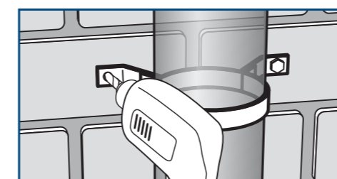
Fit bracket around existing pipework and drill through bolt holes into wall.
