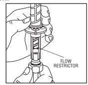
Care should be taken when installing the 400UK with a copper water supply line to prevent the copper pipe from coming into contact with the optional valve filter and/or restrictor. This may block the flow of water or cause a slow refill of the cistern.
