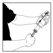
3. To adjust valve height, remove it from cistern. Twist threaded shank in or out of valve body without moving grey ring (height adjusts from 225mm. to 350mm. – the clicking noise heard is normal).
