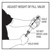
The valve height should be adjusted so that the critical level mark "C.L." on the valve is located at least 25mm. ABOVE the overflow outlet. The 400UK valve can be adjusted from 225mm. to 350mm. to fit most cisterns by TWISTING THE SHANK in or out of the valve body.
