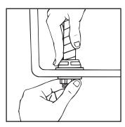
4. Position valve inside cistern and push down on the valve shank. Thread the locknut. HAND TIGHTEN ONLY. DO **NOT OVERTIGHTEN OR CISTERN MAY** CRACK. Reconnect water supply to valve. Hand tighten nut. HAND TIGHTEN ONLY. DO NOT OVERTIGHTEN OR CISTERN MAY CRACK. Make sure float moves up and down freely. IMPORTANT: See over for supply tube installation.
