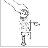
6. While holding a container over the uncapped VALVE to prevent splashing, turn water supply on and off a few times. Leave water supply off.
