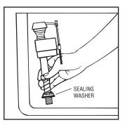
2. Place sealing washer on threaded shank and position valve in cistern, passing threaded shank through hole in cistern.
